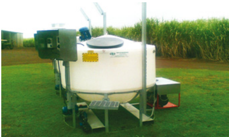
Combined Nutrigation unit with 2000L stock tank, electric agitator and electric injection unit, and control board.
