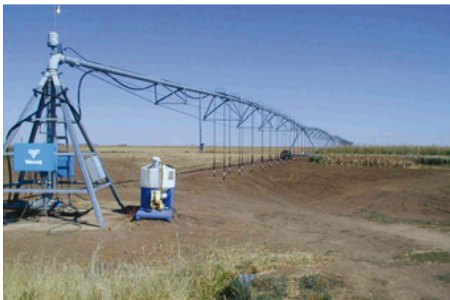
Electric driven proportional injection pump and mixing unit, including stock tank, attached to a Valley CP machine.
